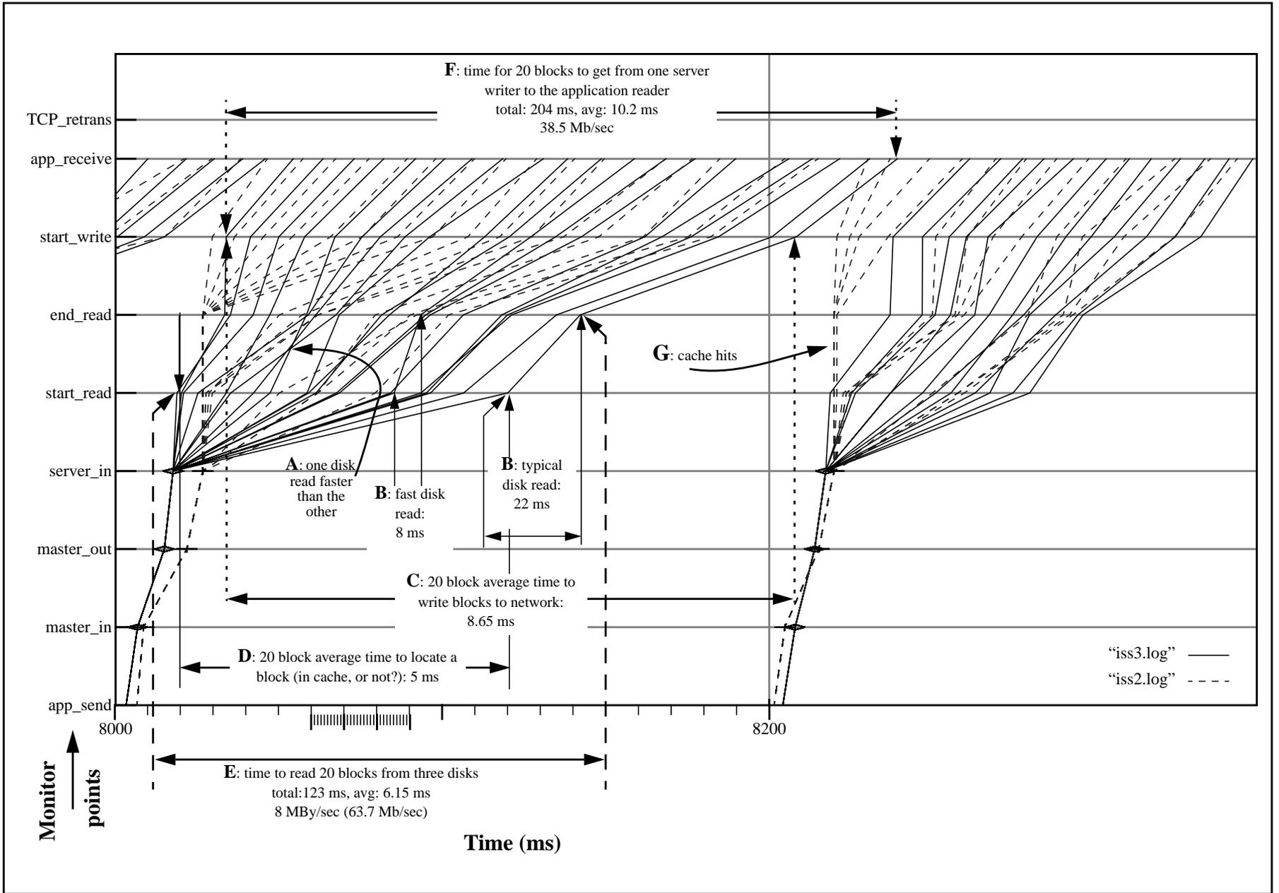
Figure 4 Detail From a Two Server, LAN, Experiment
