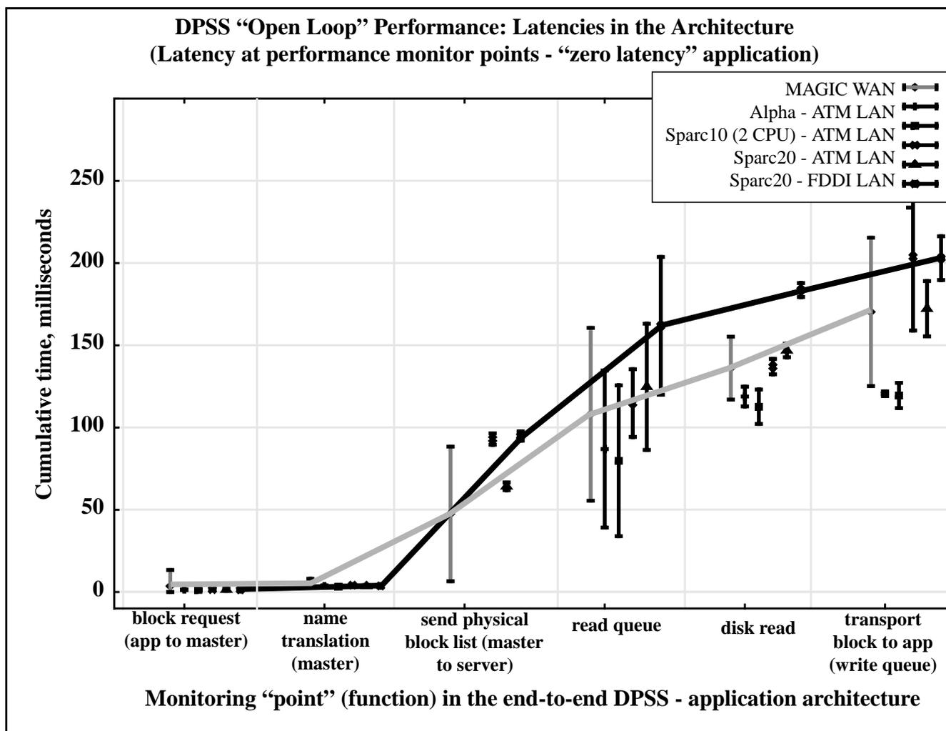
**Figure 3 Experimental Determination of Overall System Latency**
